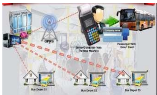
Figure 2: Architecture of city bus ticketing system
