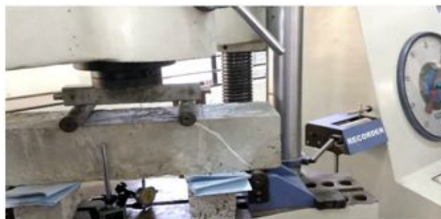
Figure 4: First cracking in S1 Specimen.
