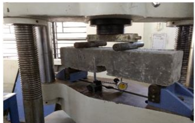
Figure 7: UTM test setup for G1 specimen.
