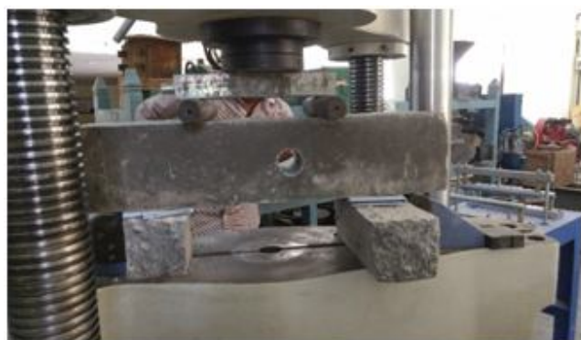
Figure 5: UTM test setup for H1 Specimen
