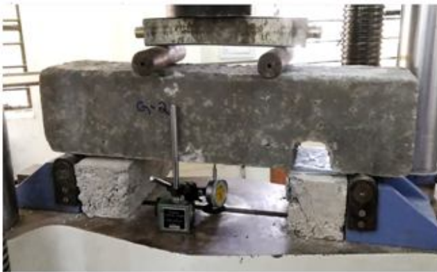
Figure 8: UTM test setup for G2 specimen
