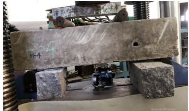
Figure 6: UTM test setup for H4 Specimen.
