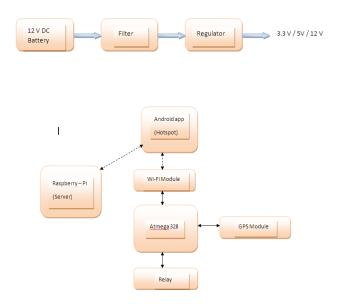
the Raspberry PI is used to create server and this Raspberry Pi is connected to android application by using wifi - hotspot. The Blynk aap is used as an android application which have ability to configure the GUI as per our project requirements. GPS is used to find the exact location of the vehicle and the co ordinates of the detected location is send to Blynk app through internet.
