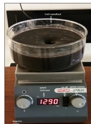
Fig: 5.2 Photographic view of \text{CuO} nanofluid preparation
