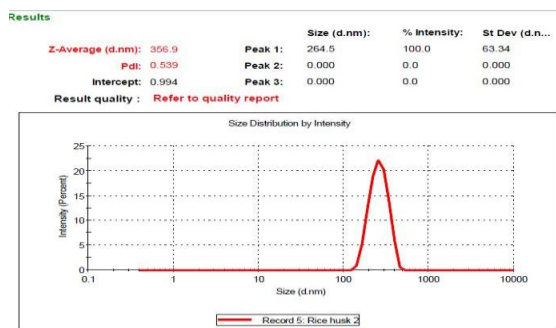
Fig 3.2. particle size result 2 hr
