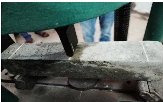
Fig 6. Centre point loading
