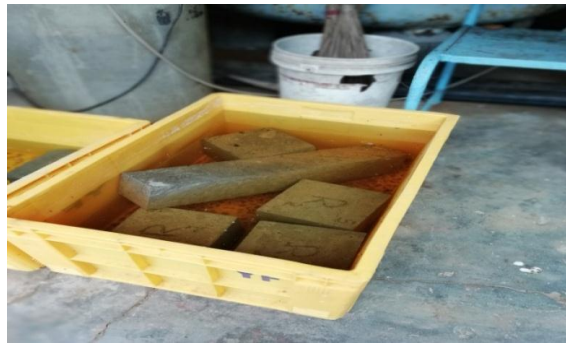
Fig 2. Curing with STP treated and reed bed treated water
