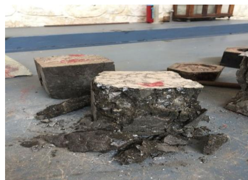
Fig 4. Failure of 7 days cube
