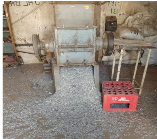
Fig1: Shredding of waste plastic
