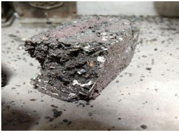
Fig 6: Eco friendly cement brick after the compression test
