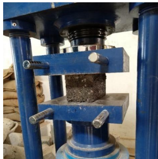
Fig 5: Eco friendly cement brick specimen being tested in CTM
