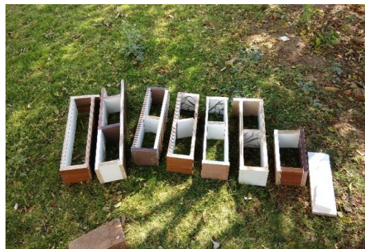
Fig 3: Ready moulds prepared from plywood waste.
