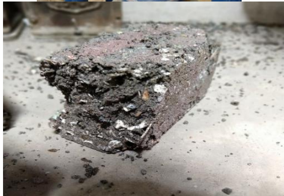
cement brick specimen being tested in CTM
