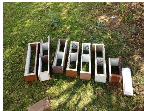
Fig 3: Ready moulds prepared from plywood waste.
