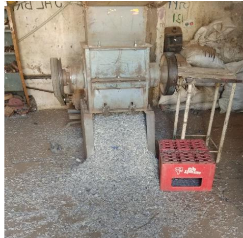
Fig 1: Shredding of waste plastic
