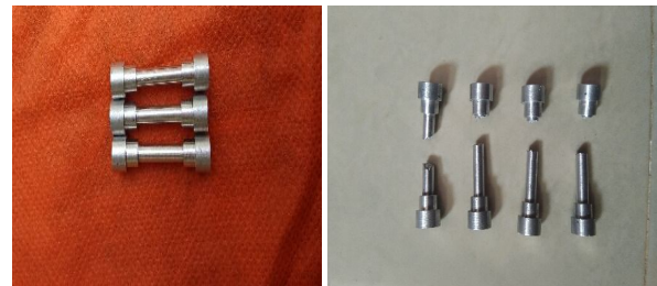
Fig : Specimens before testing Fig : Specimens after testing
