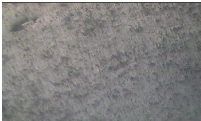
Fig.8.Microstructure of AL7075+6%SiC+3% Graphite
