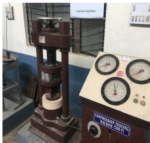
Fig 7 - Compression Test on Paver blocks
