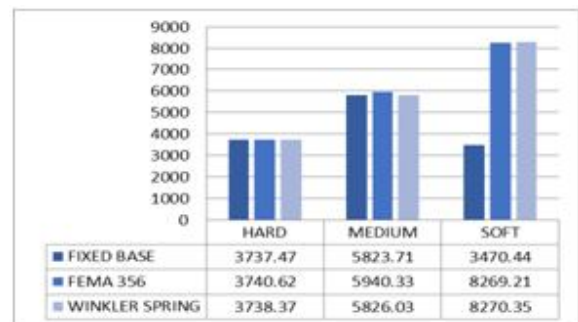
Figure 7: Base shear (kN) in X direction for RCC Frame with raft foundation
