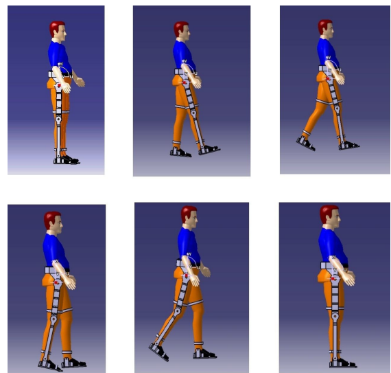
Fig.11. A series of phase of the exoskeleton walking gait cycle
