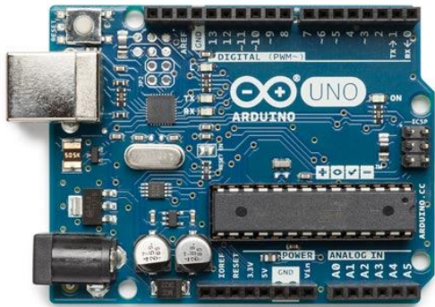
Fig 2 ARDUINO UNO Board [4]
