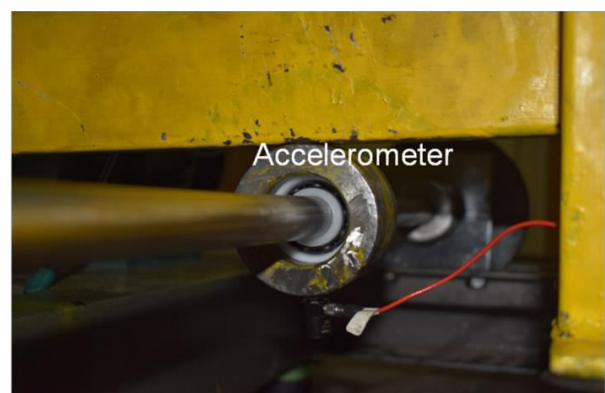
Figure 2. Bearing Housing Connected to Accelerometer
