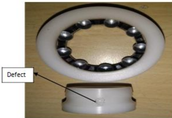
Figure 3. Defect on Ployacetal Bearing
