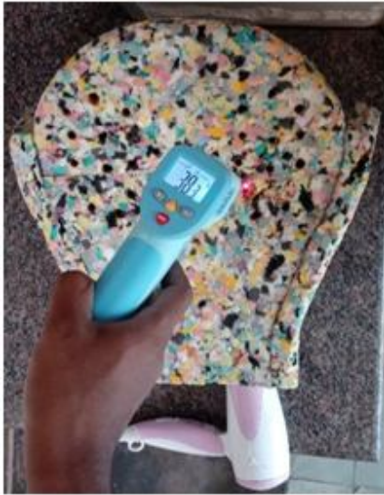
Figure 8: Temperature of seat after cooling with air blower arrangement
