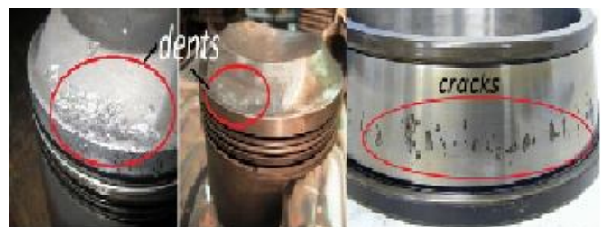
Figure 3: Defects such as Dents and cracks
