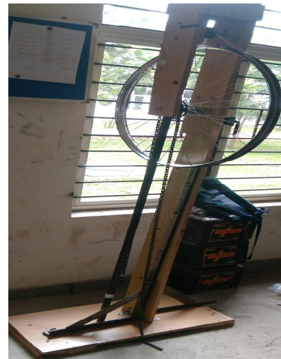
Fig.6: Fabricated gravity powered light
