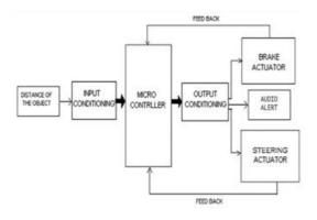
The system detects the distance of obstacle at various stages and gives output response as programmed at a various level which could be audio, visual or mechanical action or combination of all.
