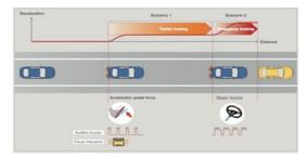
At this, Distance from the front obstruction will be set as a parameter. This will work in stages were the first action will act as passive driver alert system which will only warn the driver about obstruction directly in line with the path of the vehicle. Here only an audio alert will be given to the driver about the obstruction ahead as could be seen in fig 3.1.
