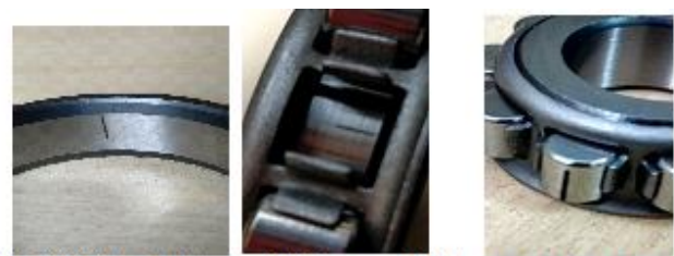
Fig 2.2(i) Outer defect
