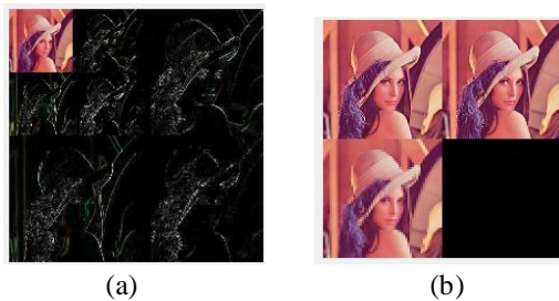
Fig 3: (a) Second level decomposition of the image Lena with in image. (b) Decomposed image with the out space after quantization of required energy.
