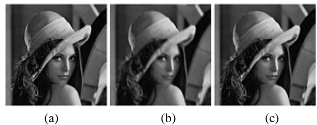
Fig 8: CS-based Shrinkage Image Reconstruction. (a) Original Lena Image of dimension [0,256] (b) Noised image (c) Reconstructed Image.
