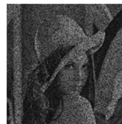
Fig 6: Lena image captured with PCI Matrix with 50% sampling ratio and the zero is been used to the place where the samples is not been captured.
