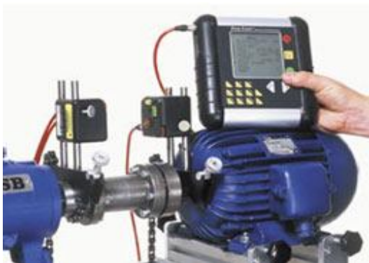
Fig. Alignment with laser equipments
