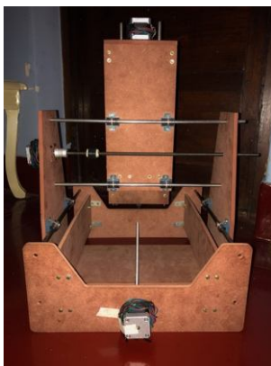
Figure 3: Rear view of the assembly of the building frames, lead screws and stepper motors.
