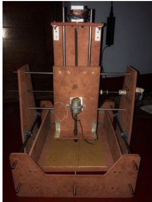
Figure 2: Front view of the assembly of the building frames, lead screws and stepper motors.
