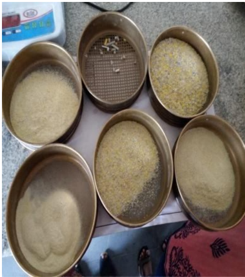
Figure: 7 Sieve analysis of pulverized plastic
