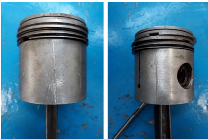
Fig.6 Scratched (Faulty) piston
