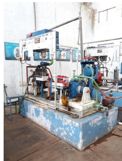
Fig. 1 Four-stroke four-cylinder petrol engine.
