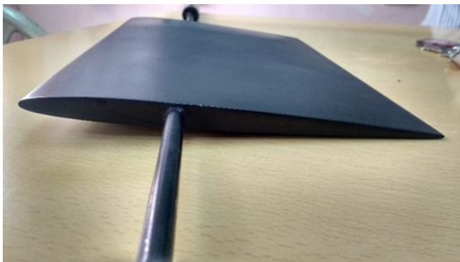
Figure 6: Fabricated model of NACA 0006
