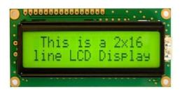
A liquid-crystal displays flat display which uses light-modulating properties of liquid crystals. Backlight or reflector is used to produce images.
