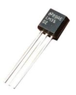
Temperature sensor LM35 is a commonly used sensor. Temperature sensor is used to measure temperature with electrical output comparative to the input temperature. It will measure temperature greater efficiently as compared with a thermistor.
