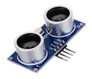
An Ultrasonic sensor is a tool which could degree the gap to an item by the use of sound waves. It measures distance through sending out a sound wave at a particular frequency and listening for that sound wave to get better. Ultrasonic sensors are used for the obstruction avoidance since it is the efficient sensor for detecting the limitations.
