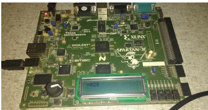
Fig. 6.3 DA output1 displayed on LCD on Spartan 3E board
