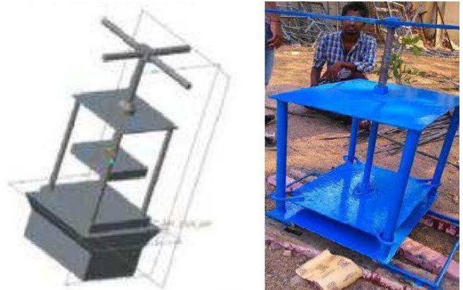
Fig3: Screw Press Design and Fabricated Model
