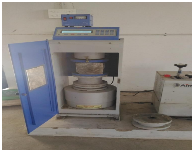
Fig : Compressive strength testing machine
