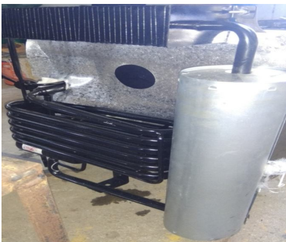
Figure-8 Experimental set up of Vapour adsorption system
