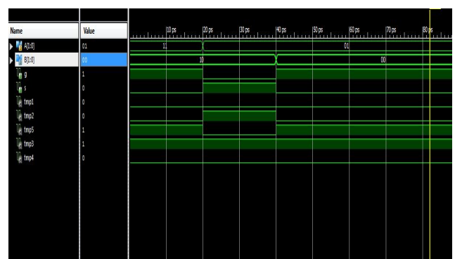
Figure 7. (a) Waveform showing input output of 2-bit comparator
