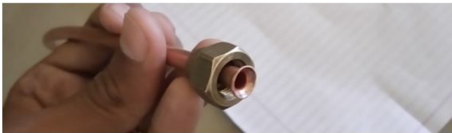
Fig. 5. Flared copper tube along with flare nuts [15]
