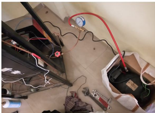
Fig. 3. Evacuation or air removal [15]
