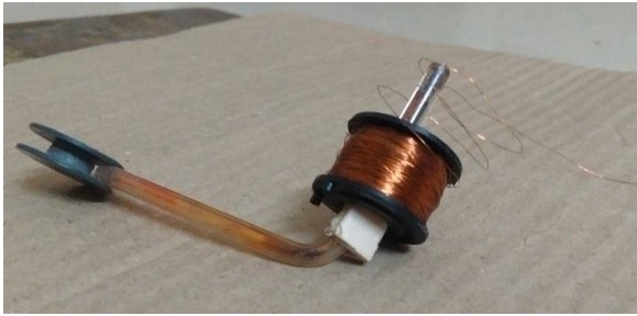
Figure 4 Sensor (Disk with capillary and coil )
