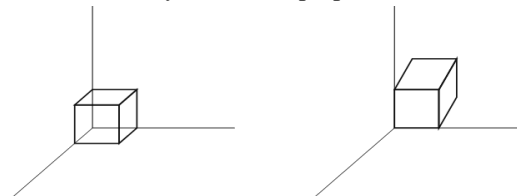
Fig.38: A Unit Cube a) is sheared b) by transformation matrix a = b = 1
