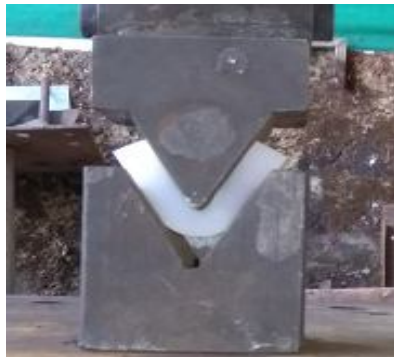
Figure 4: Actual experimental set up for v-bending
