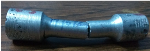
Figure 5 Tensile Test Specimen Sample-B (A356-91%, E-Glass fiber-3% and Fly Ash-6%)
