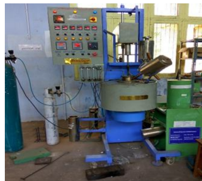
Figure 1 Stir Casting Setup
