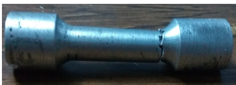
Figure 6 Tensile Test Specimen Sample-C (A356-88%, E-Glass fiber-3% and Fly Ash-9%)
