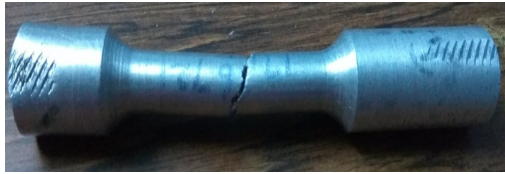
Figure 4 Tensile Test Specimen Sample-A (A356-100%)
