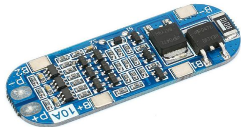
Figure 6. 18650 Lithium battery protection module
