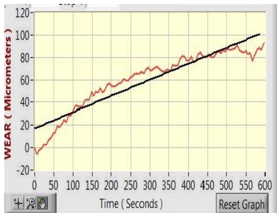
Figure 7 Wear behavior of heat treatment (400°C) and oil quenching sample
