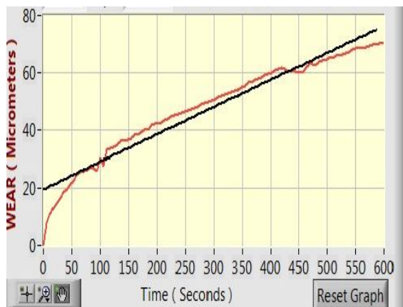
Figure 8 Wear behavior of heat treatment (500°C) and oil quenching sample
