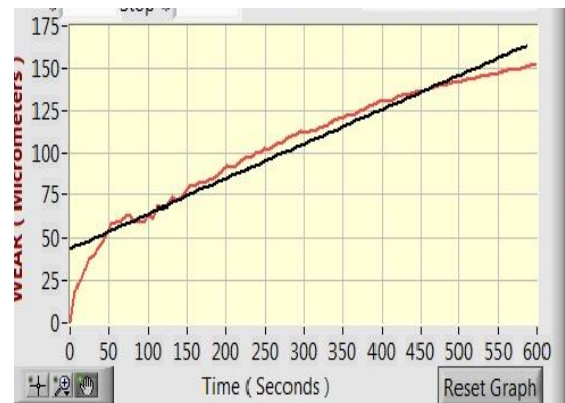
Figure 4 Wear behavior of heat treatment (300°C) and air quenching sample
