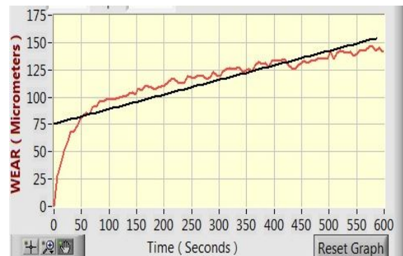
Figure 5 Wear behavior of heat treatment (300°C) and water quenching sample
