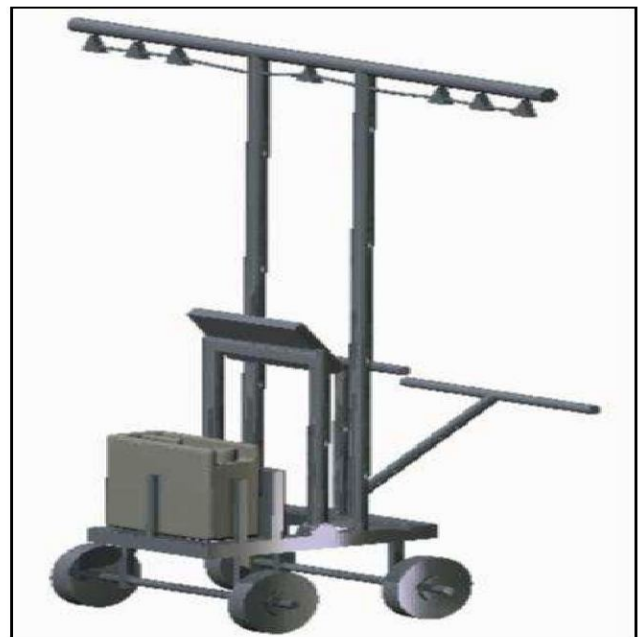
Figure 2. Trolley Based Solar Operated Pesticide Sprayer.
