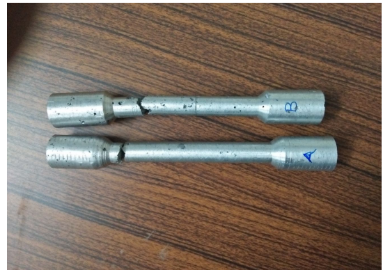
Figure 5.3 Tensile specimen after failure
