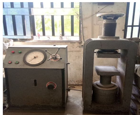
Fig 1 : showing testing of compressive strength
