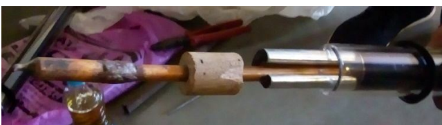
Heat pipe assembly inside glass tube with fin (At SSPM's COE, Kankavli, 10/04/2018)
