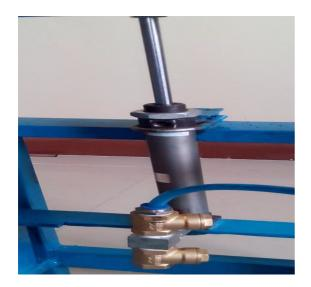
**3.** Swing type check valve (NRV): The swing type check valve is used for supply the air from cylinder to the air tank for the storage purpose. It allows the fluid flow in only one direction. The main advantage of swing type check valve is it operates on minimum upstream pressure.
