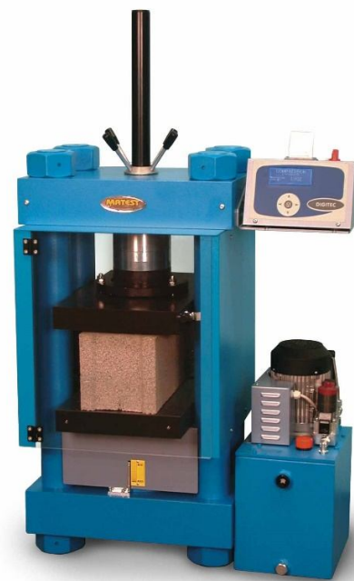
Fig 3: compressive strength test
