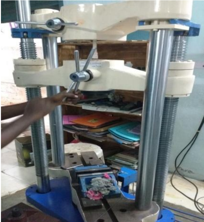
Fig. 2.5 UTM machine sample loading condition for tensile test
