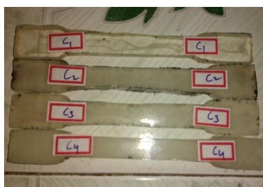
Fig.2.2 Tensile test specimens before Test
