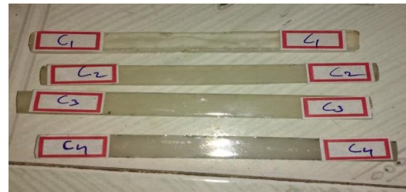
Fig.2.3 Flexural test specimens before Test
