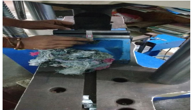
Fig 2.6 Sample loading condition for 3 point bending test
