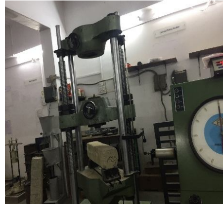
Fig 4 Testing setup of UTM
