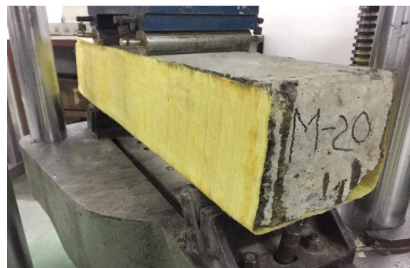
Fig 6 Two point load for Flexural test after retrofitting using AFRP Sheet.
