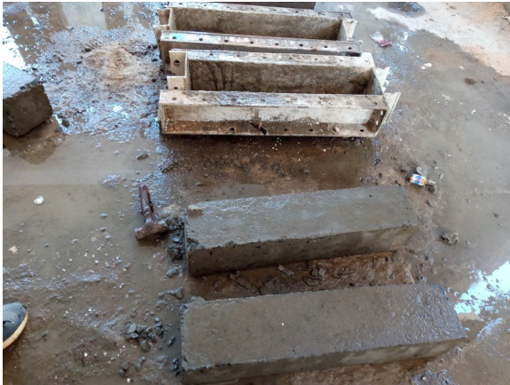
Fig 1 De-moulding of beam.
