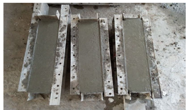
Fig 1 Casting of beam.
