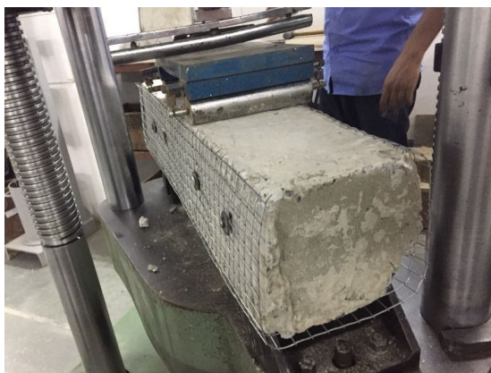
Fig 9 Two point load for Flexural test after Retrofitting using wiremesh
