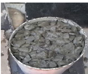
Figure: Casting of cylinder in PVC pipes
