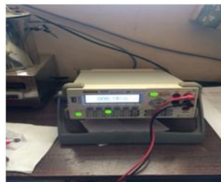
Fig 8: Testing of Electrical Resistance by Multimeter
